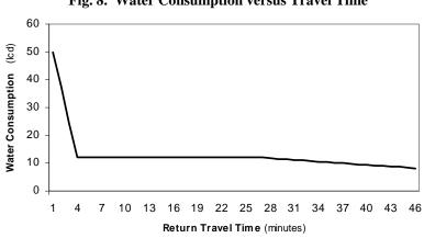
Fig. 8. Water Consumption versus Travel Time
