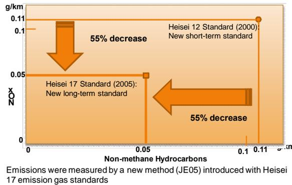
**Figure B: Diesel Vehicle's Emission Standard in the Heisei 17 Emission Standard**
