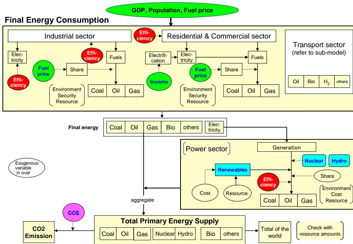
Figure 2-1 Flowchart of the IEEJ2050 Model
